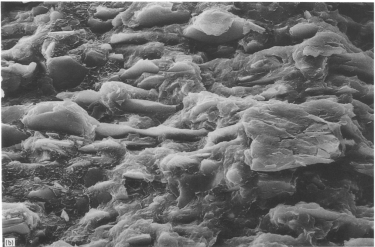
Figure 13 Scanning electron micrographs of glass/polyethylene composite fracture surface with (a) 20 vol% unmodified mica and (b) 20 vol% mica modified with 1 equivalent molecular layer of azido-functional silane.
